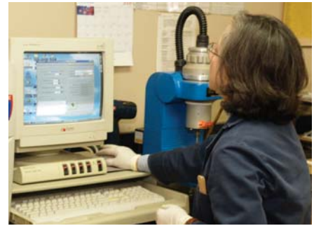
Martin Asphalt lab tests dynamic shear rheometry.
