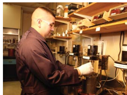
Measuring asphalt viscosity in the lab.
